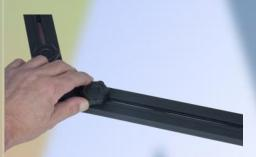
9. Adjust the spreader so that the legs are at the desired angle by loosening the spreader adjustment knob and then retighten it.
