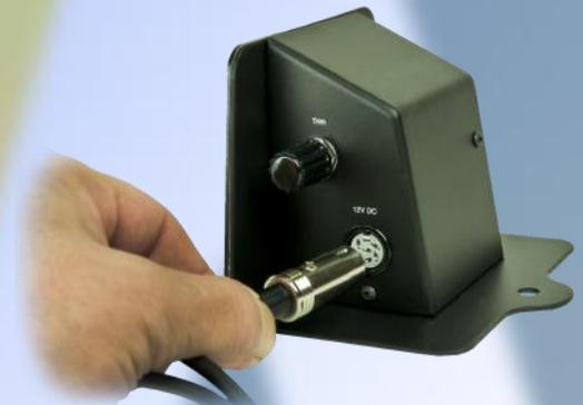
7. To supply power to the Cue Light, plug the power cord into the socket marked 12V DC.
