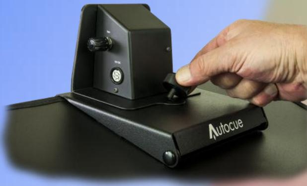
4. Re-secure the hood frame retainer. The Cue Light is now mounted to the hood.
