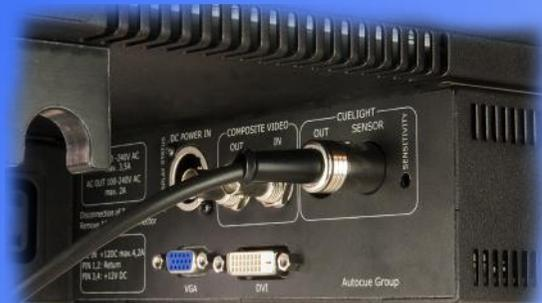
9. Plug in the power cable into the sensor socket. This will provide power to the cue Light. This socket is only available on the MSP range of monitors.
