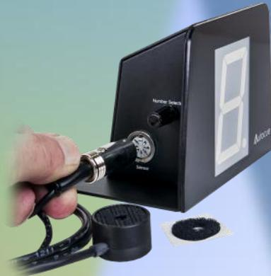
6. To install the sensor, plug the unit into the socket marked sensor.
