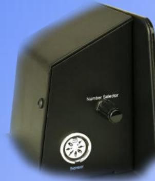
11. Rotate this control until the desired camera number is displayed.
