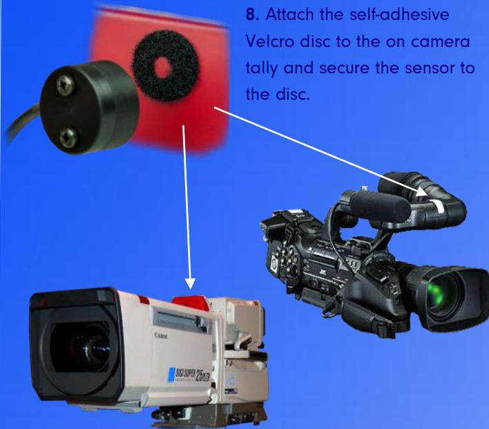
8. Attach the self-adhesive Velcro disc to the on camera tally and secure the sensor to the disc.
